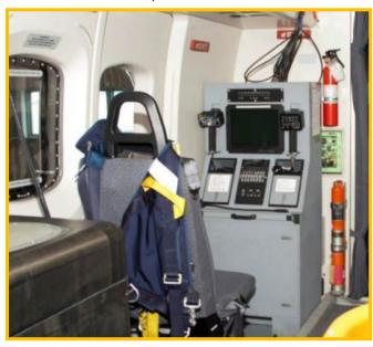
Platform serves as locator tracking screen, FLIR and Nitesun control, communication hub: radios, SAT phone and medical triage relay to onshore emergency physician.
